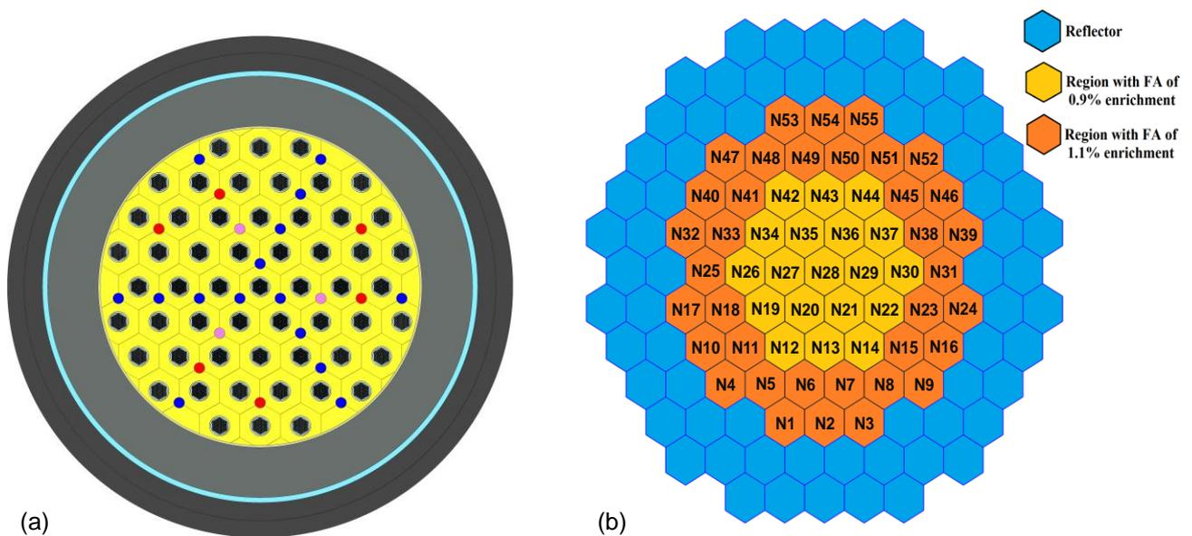
Figure 1: (a) TEPLATOR reactor core with control rods (pink represents regulating rod, blue represents compensation rods and red represents emergency rods), (b) reactor core nodalization with different enrichments.
