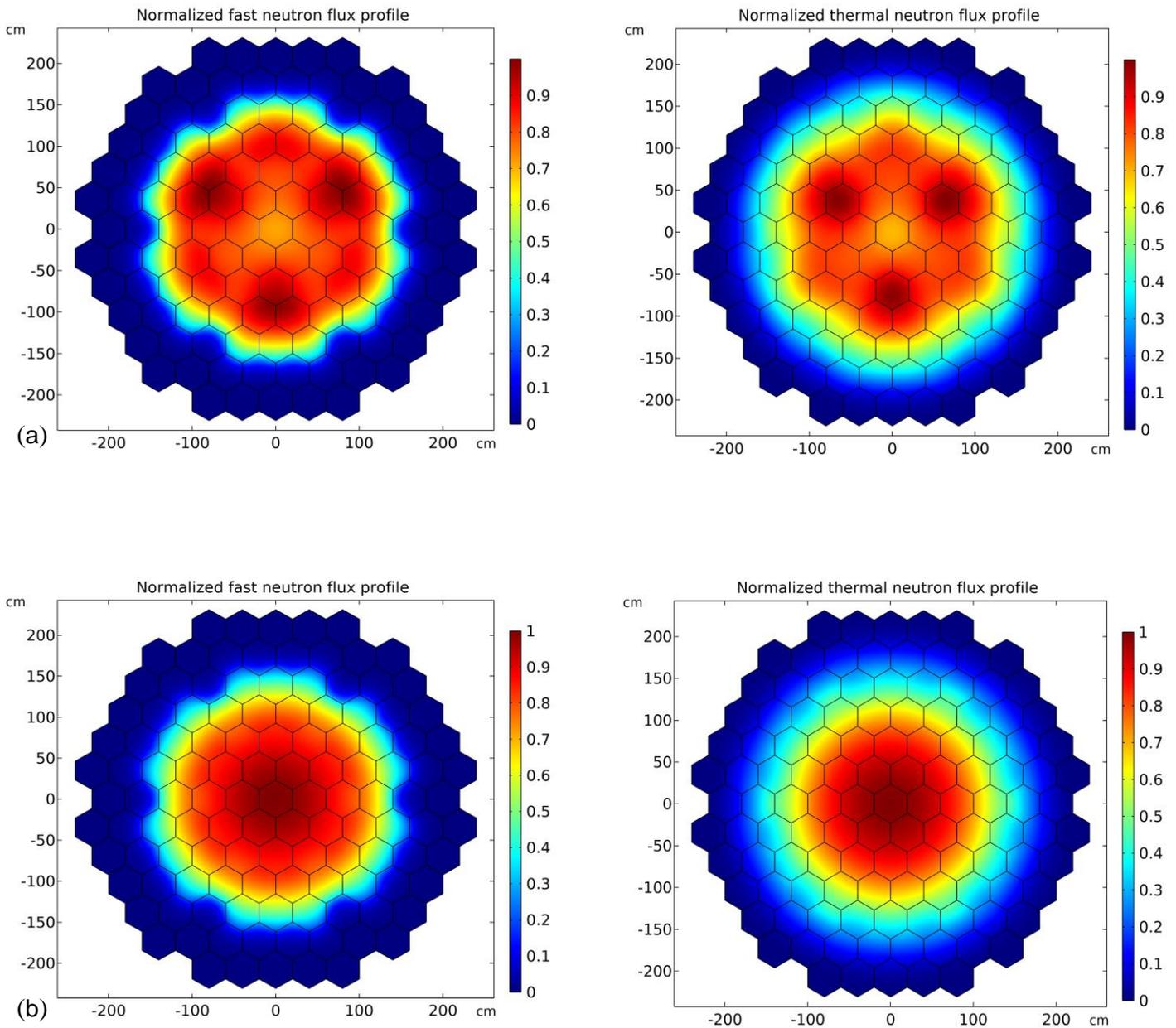
Figure 3: Normalized fast and thermal flux profile for BOC (a) case 1 (All the rods are inside the reactor core) (b) case 2 (All the rods are outside the reactor core).
