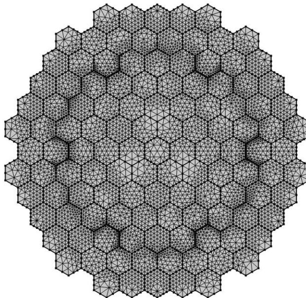
Figure 2: Two-dimensional mesh structure generated by COMSOL for the Teplator core.
