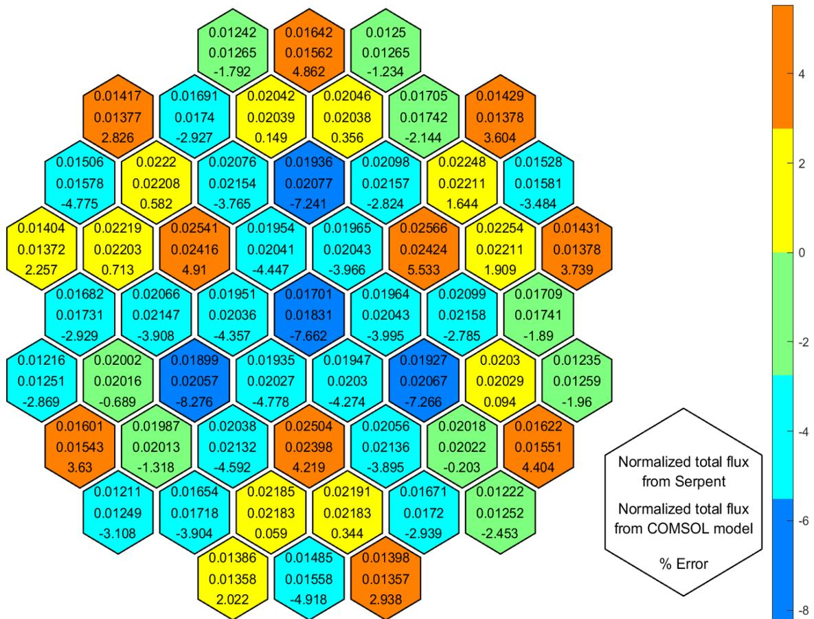
Figure 4: Normalized total flux distribution (normalized to 1) in hexagonal cell calculated from COMSOL diffusion model and Serpent code, for case 1 BOC.
