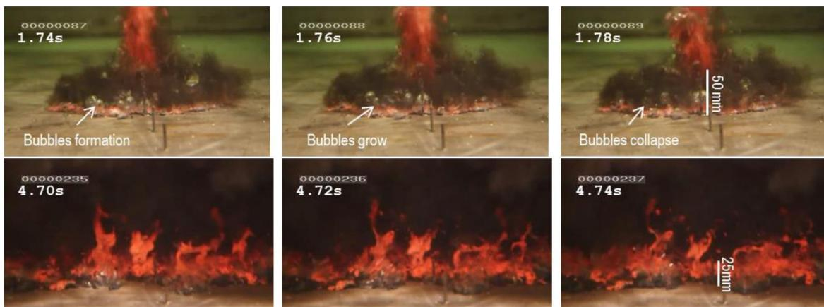
Figure 1: Melt jet and melt spreading with the formation of the premixed layer in the PULiMS-E4 experiment. The figure is adopted from [5]
