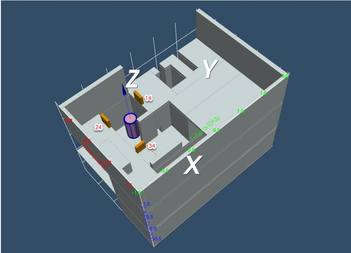
Figure 2: HI-TRAC in decontamination area in FHB and used tally locations
