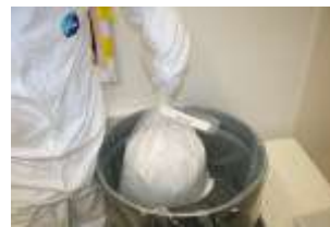
Figure 9: Solidified waste package
