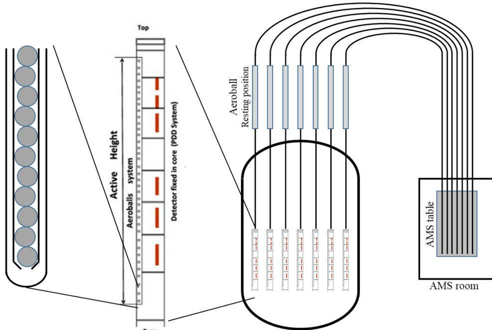
Figure 1: Schematic view of the AMS components. Left: Aeroball guide tube with ball stop (permeable to carrier gas). Center: Schematic view of a fuel assembly with AMS probe. Right: Total view of the AMS
