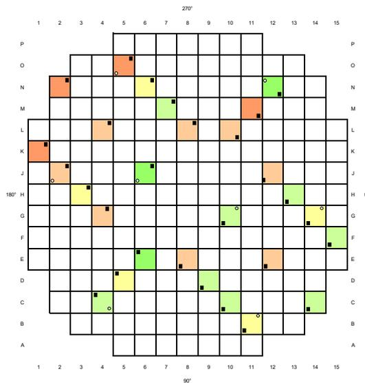
Figure 2: Distribution of the AMS probes in a Siemens/KWU built 1300 MW PWR
