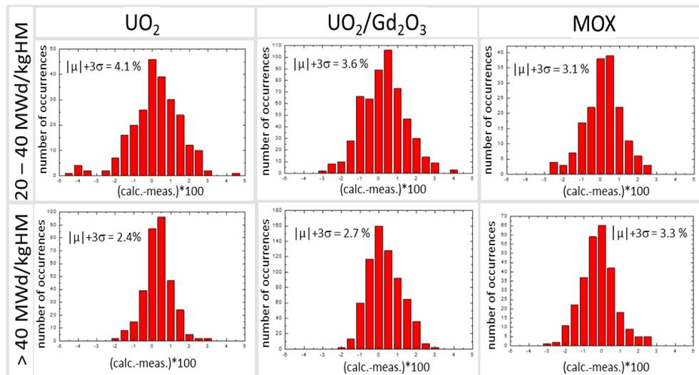
Figure3: Distribution of the differences calculation–measurement of the fuel burnups for different fuel types and burnup intervals
