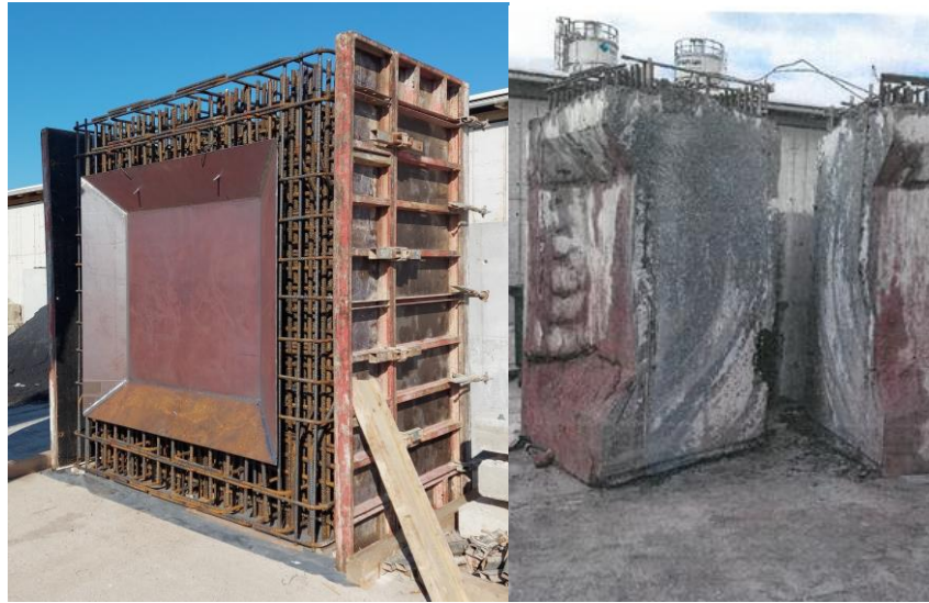
Figure 3: Rebar cage of part of primary wall (left) and the concrete blocks of primary wall cut on half (right).
