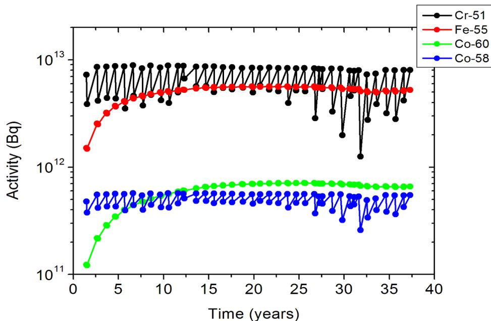
Figure 4: Time course of some nuclide activities calculated with ORIGEN for the steel of a core shroud in a PWR which was irradiated for approximately 37 years.
