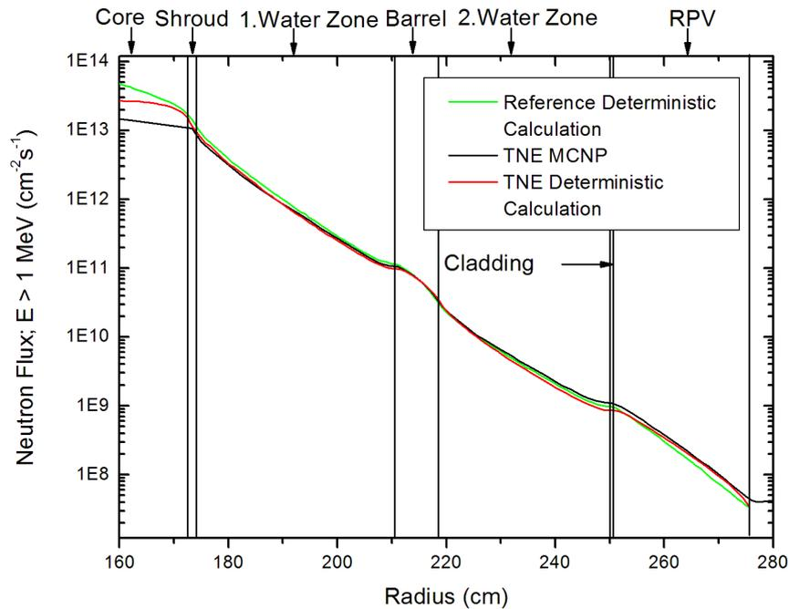
Figure 4: Comparison of fast neutron fluxes ( $E > 1 \text{ MeV}$ ) calculated with a deterministic code and MCNP.
