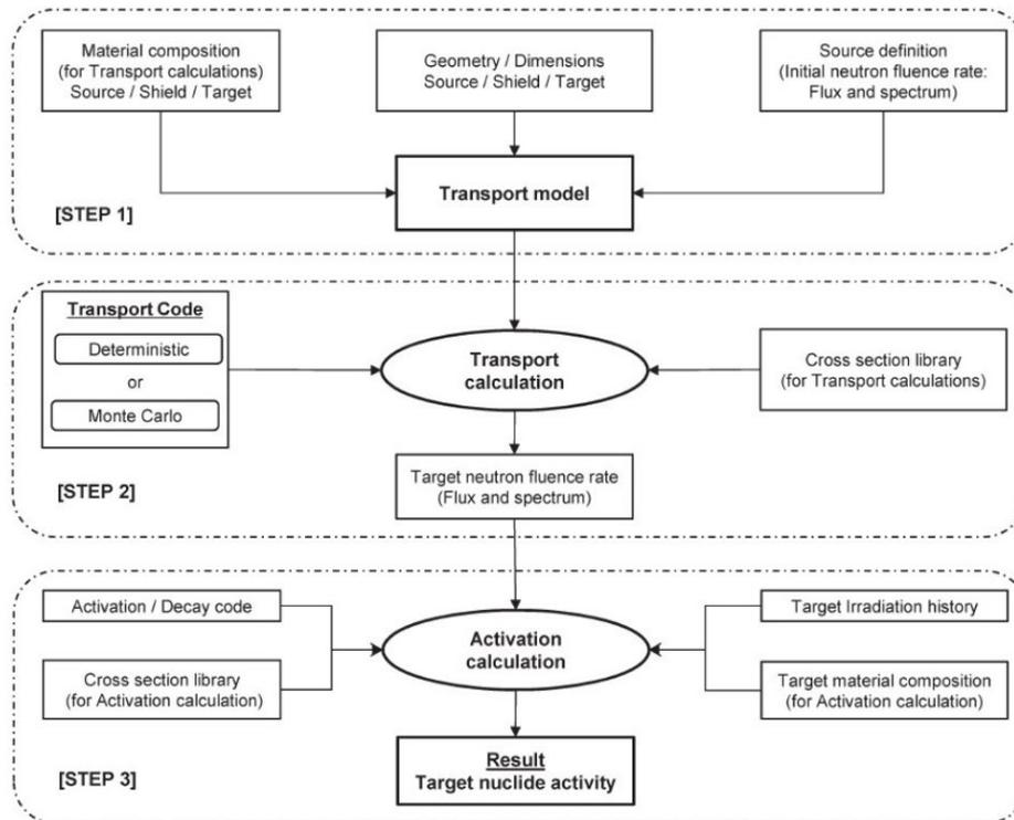
Figure 1: Flowchart of the calculation procedure (referred to [3]).
