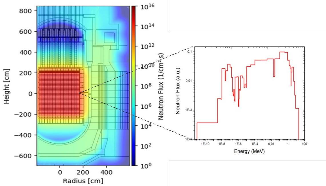
Figure 2: Mesh-Plot of the total neutron flux in the core center plane of a PWR and the corresponding neutron flux spectrum of the core shroud in a 56-energy group structure.
