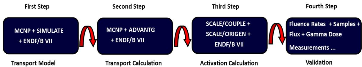
Figure 3: Scheme of the calculation procedure used by TNE to calculate activation activities.
