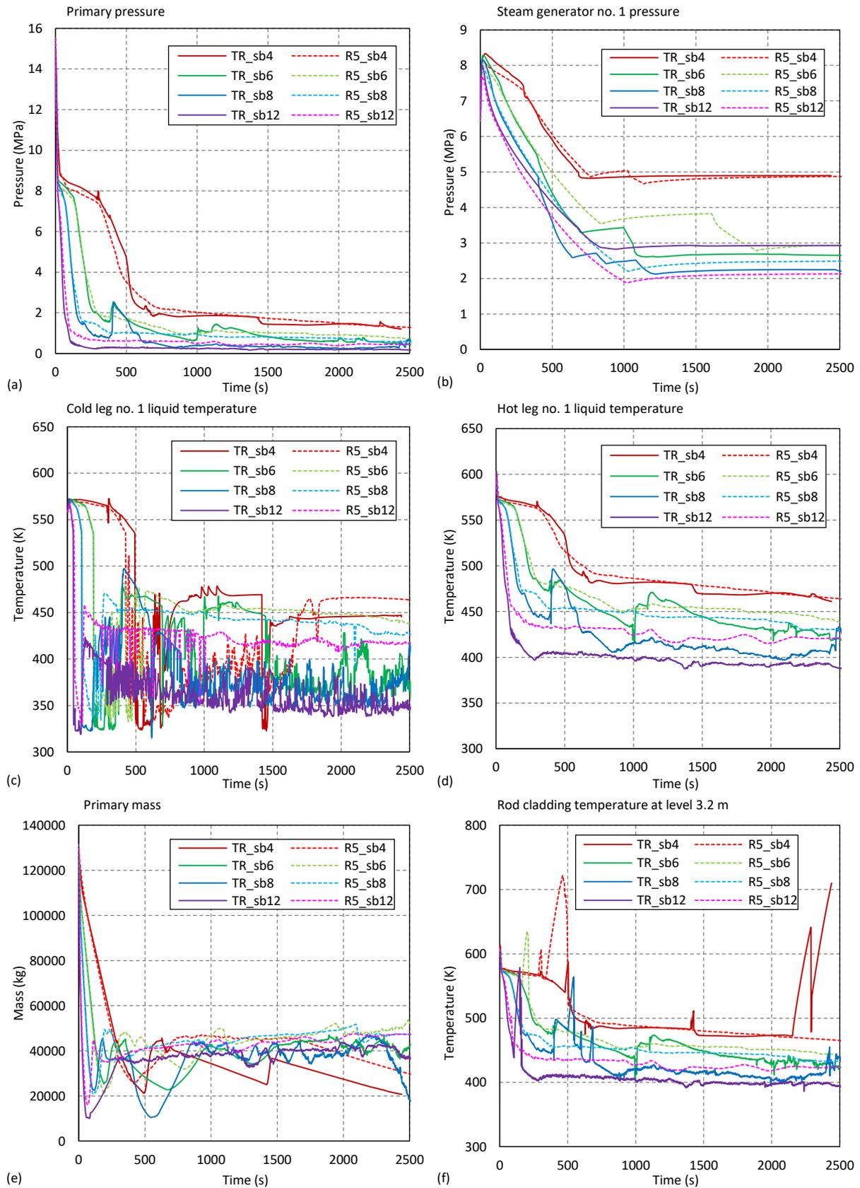
Figure 3: Comparison between TRACE and RELAP5 for 10.16 cm, 15.24 cm, 20.32 cm and 30.32 cm break size LOCAs (part 1)
