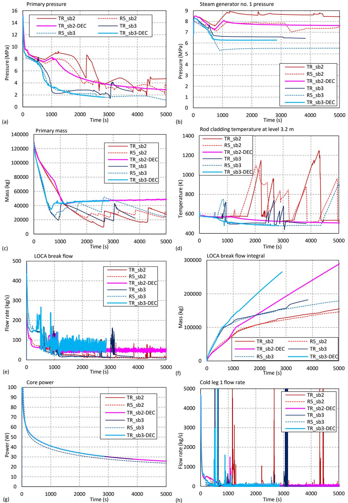
Figure 2: Comparison between TRACE and RELAP5 for 5.08 cm and 7.62 cm break size LOCAs
