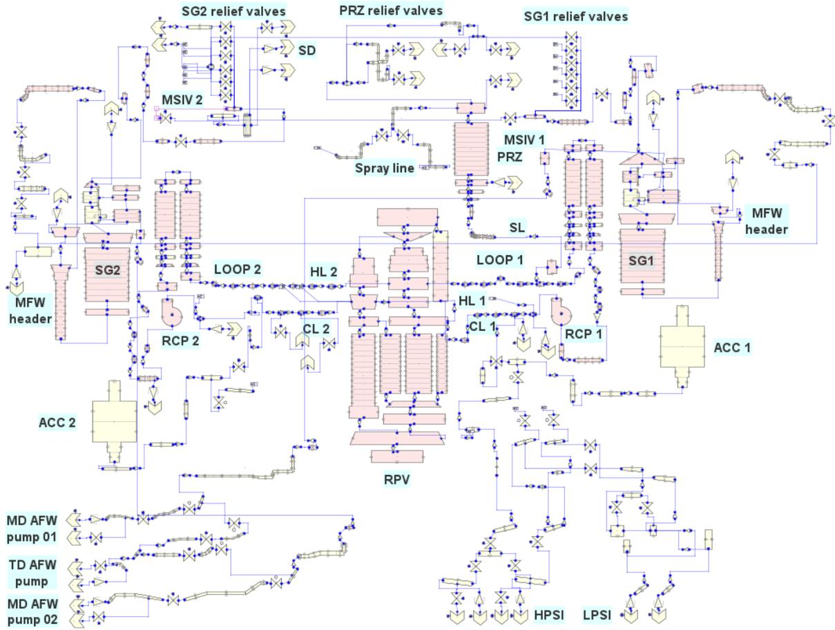
Figure 1: TRACE two-loop PWR hydraulic components view
