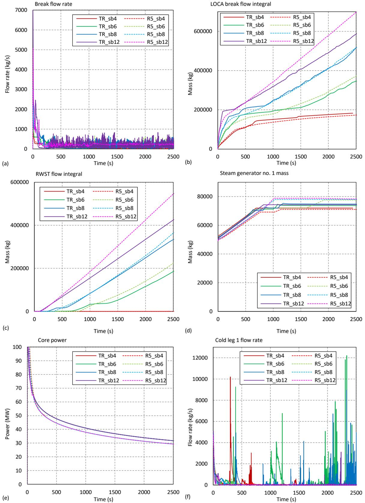
Figure 4: Comparison between TRACE and RELAP5 for 10.16 cm, 15.24 cm, 20.32 cm and 30.32 cm break size LOCAs (part 2)
