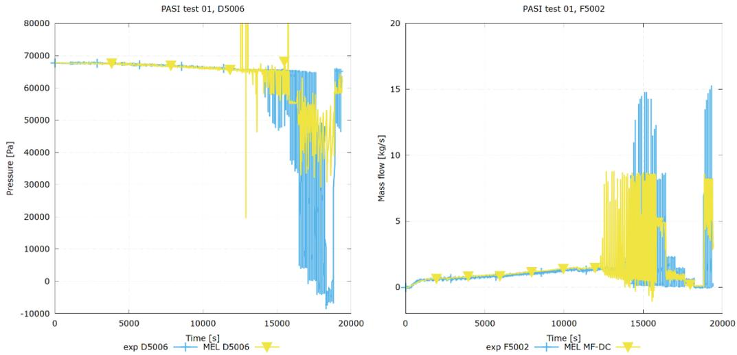
Figure 6: MELCOR results of the PAS-01 (left – pressure difference across the downcomer, right – mass flow in the downcomer)
