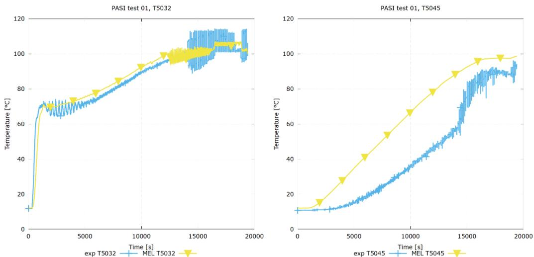
Figure 7: MELCOR results of the PAS-01 (left – temperature in the riser, right – temperature in the pool)
