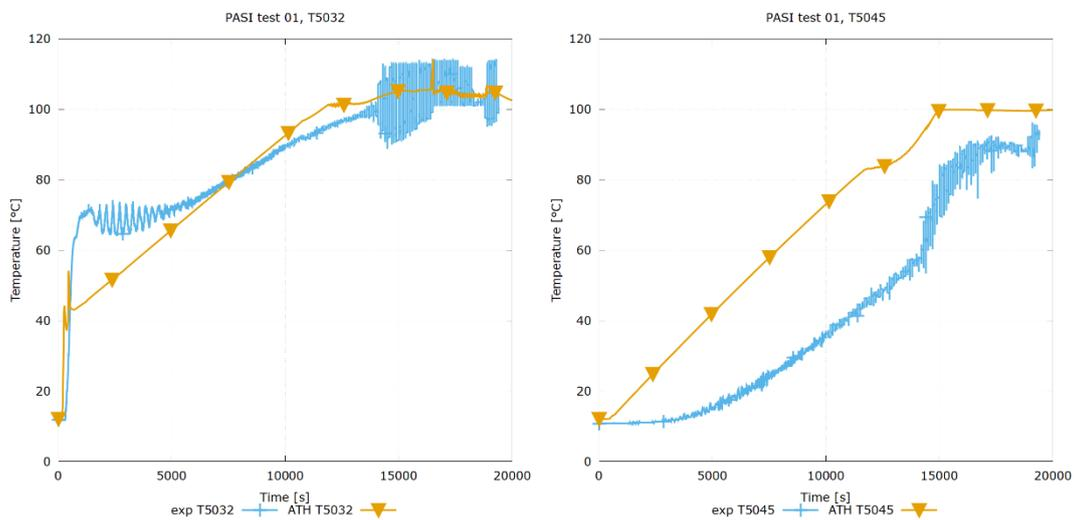
Figure 4: ATHLET results of the PAS-01 (left – temperature in the riser, right – temperature in the pool)
