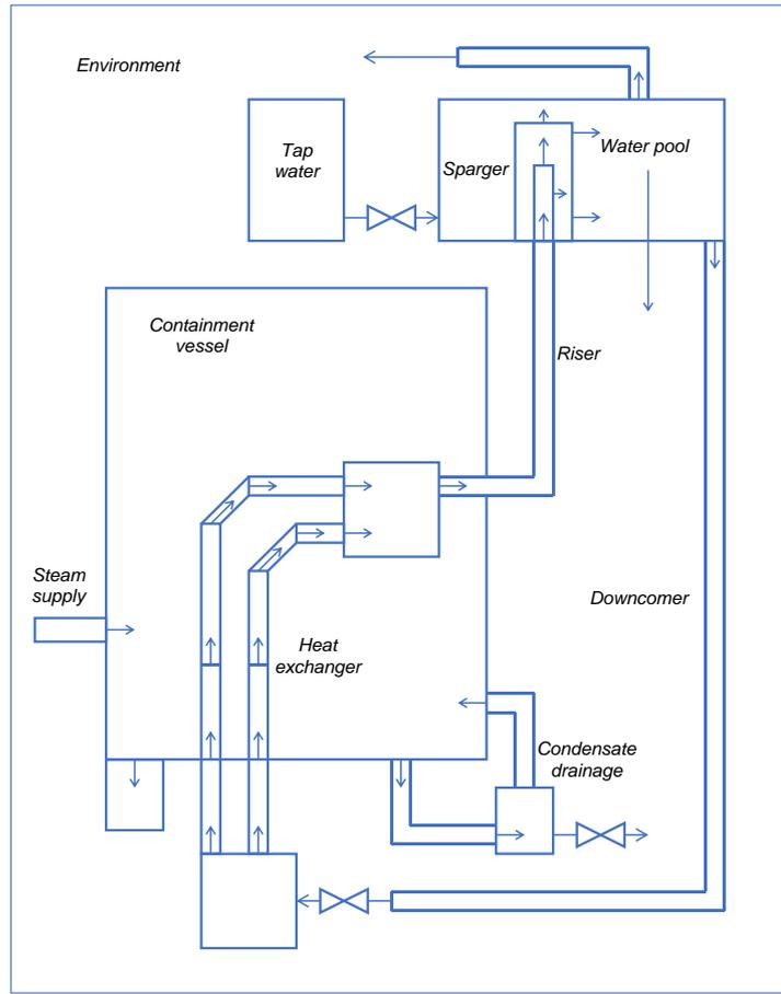
Figure 5: MELCOR nodalisation of the PASI test facility
