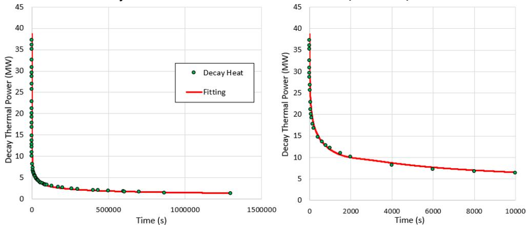
Figure 2: Decay heat power curve and its fitting imposed as boundary condition to perform the CFD analyses [4].
