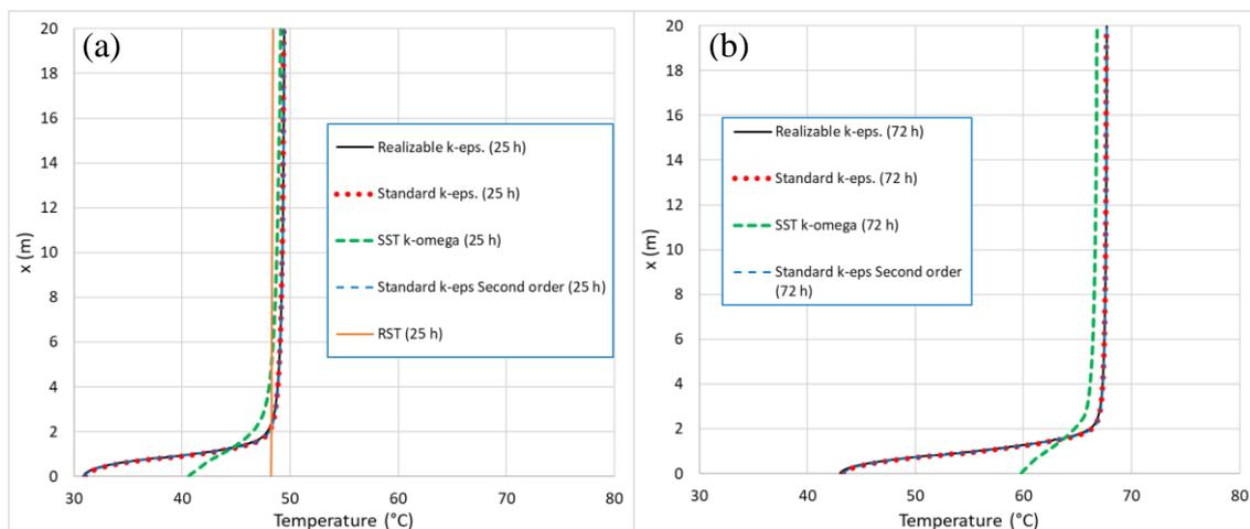
Figure 5: temperature behaviour along a vertical section of the pool achieved with different turbulence models at two reactor times: (a) 25 h; (b) 72 h.
