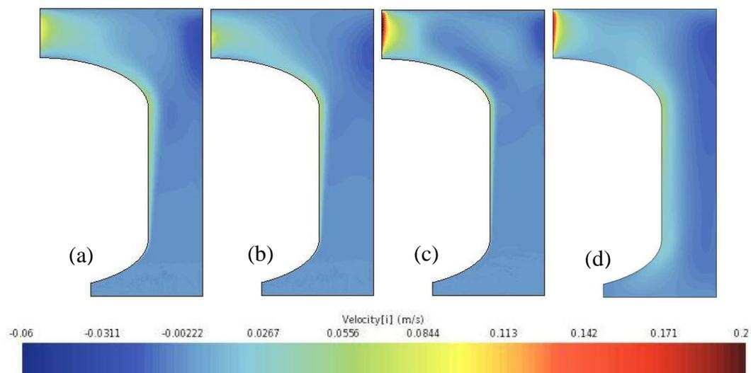
Figure 4: vertical velocity field (in m/s) achieved in the cooling pool after 25 hours of simulating time with different turbulence models: (a) Standard  $k-\epsilon$ ; (b) Realizable  $k-\epsilon$ ; (c) SST  $k-\omega$ ; (d) RST transport model.
