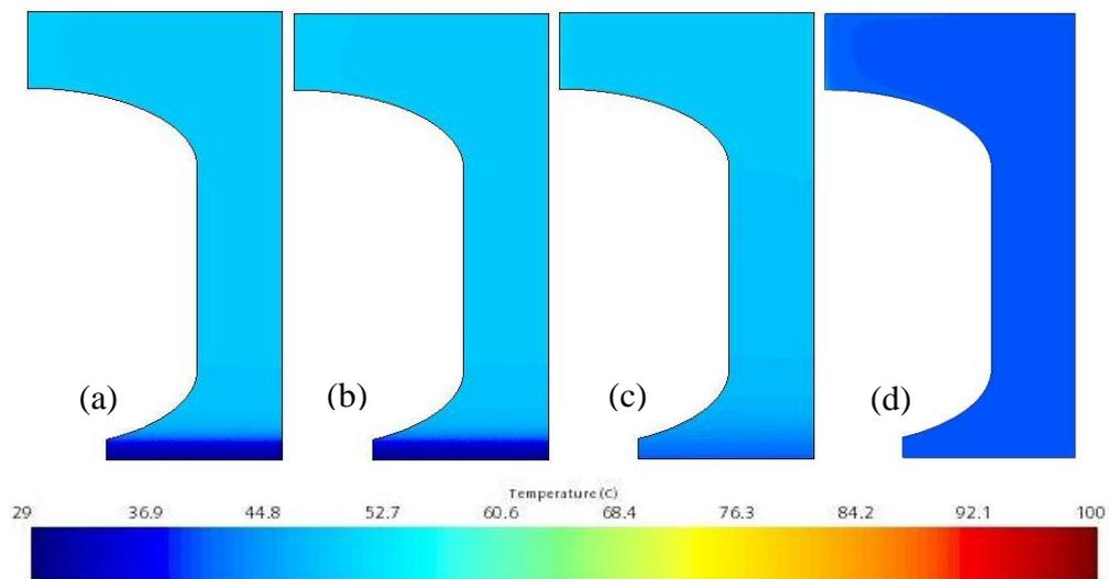
Figure 3: temperature field achieved in the cooling pool after 25 hours of simulating time with different turbulence models: (a) Standard  $k-\epsilon$ ; (b) Realizable  $k-\epsilon$ ; (c) SST  $k-\omega$ ; (d) RST transport model.
