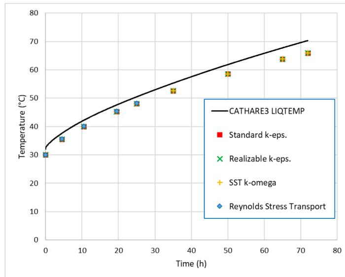
Figure 6: Comparison between CFD mass averaged temperature and CATHARE3 results.
