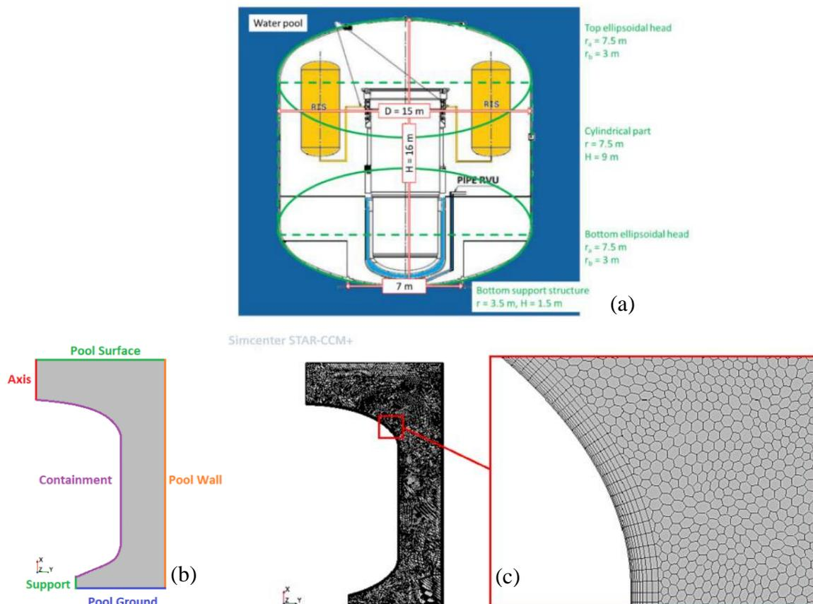
Figure 1: Computational domain with a sketch of the modelled system (a), the boundaries (b) and a portion of the generated mesh adopted in the CFD analyses (c) [4].
