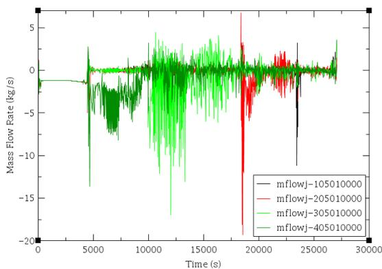
Figure 5. Mass flow rates in the four hot legs in case A
