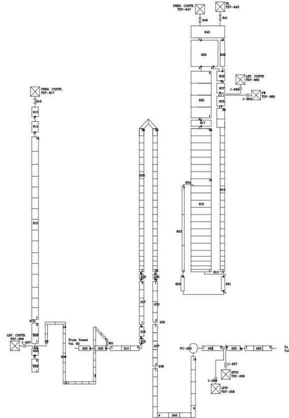
Figure 4. Loop 2 and SG secondary side nodalization, 1 U-tube SG
