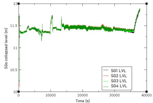
Figure 8. Steam generators collapsed level in case B
