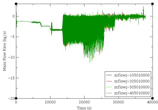
Figure 7. Mass flow rates in the four hot legs in case B
