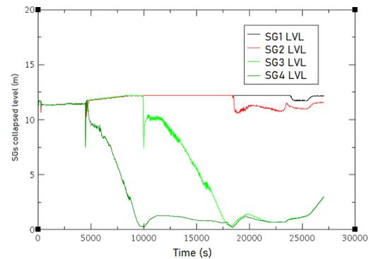
Figure 6. Steam generators collapsed level in case A
