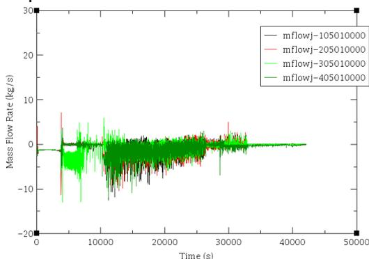
Figure 13. Mass flow rates in the four hot legs in case E
