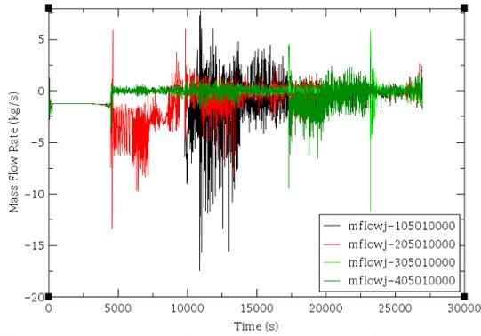
Figure 9. Mass flow rates in the four hot legs in case C
