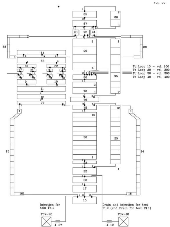
Figure 3. Reactor pressure vessel nodalization
