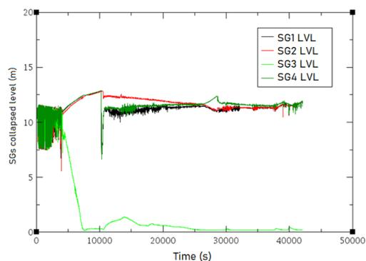
Figure 14. Steam generators collapsed level in case E
