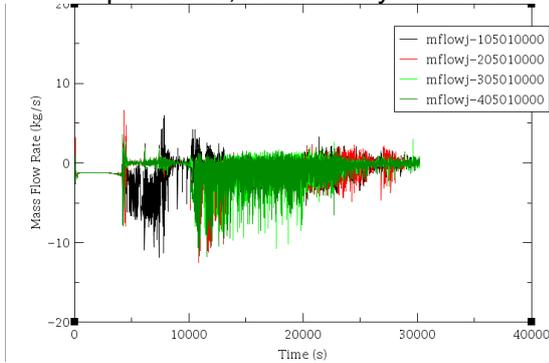
Figure 11. Mass flow rates in the four hot legs in case D
