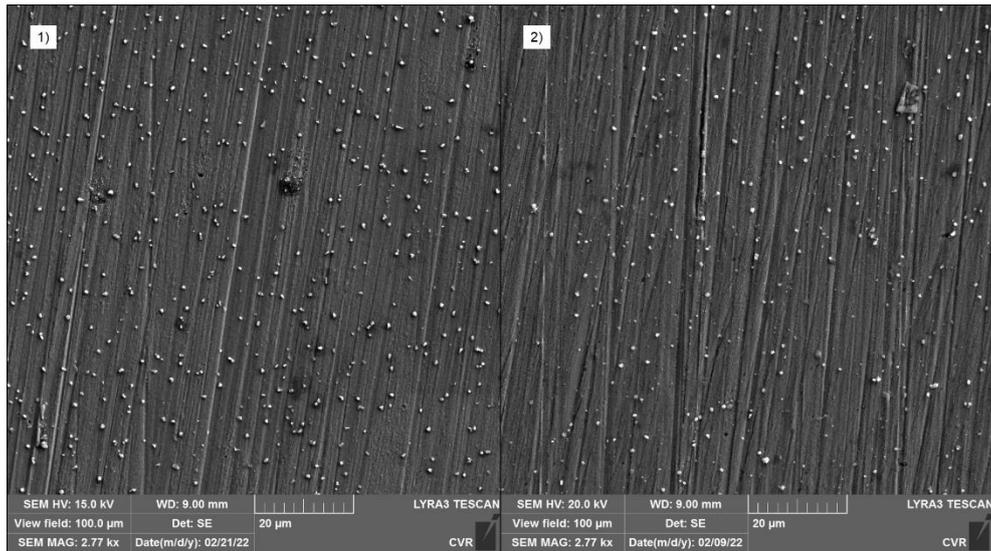
Figure 3: Surface of 1) 800H, and 2) 316L after exposure (by SEM, SE, MAG 2.77 kx)
