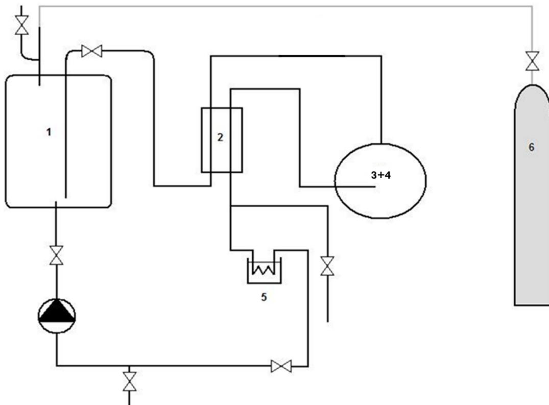
Figure 1: Scheme of an experimental device for SCW environment. 1) demineralized water tank 2) heat exchanger 3+4) high-temperature autoclave with heating and internal sample space 5) water cooling 6) argon pressure vessel [6].
