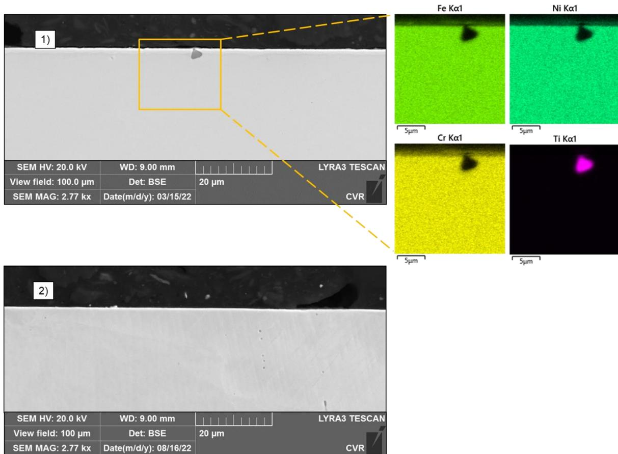
Figure 4: Cross-section of 1) 800H with elemental maps 2) 316L after exposure (by SEM, BSE, MAG 2.77 kx)
