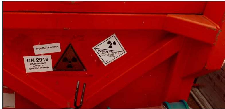
Figure 2: A type B package with Category 2 radioactive source (source of photo: SNSA)
