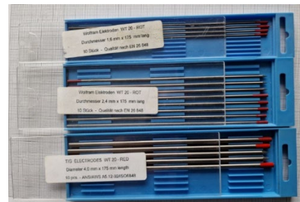
f – Welding electrodes containing Th-232
