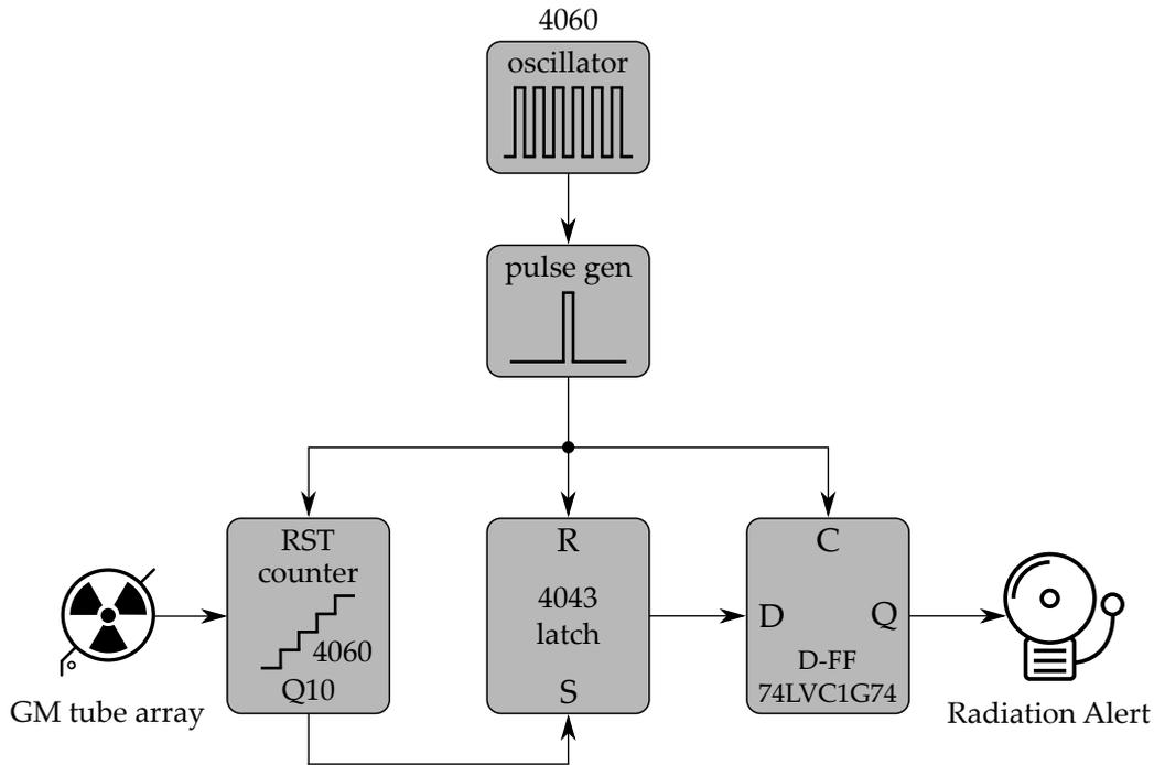
Figure 3: Block diagram of the proposed radiation tolerant pulse counter circuit.
