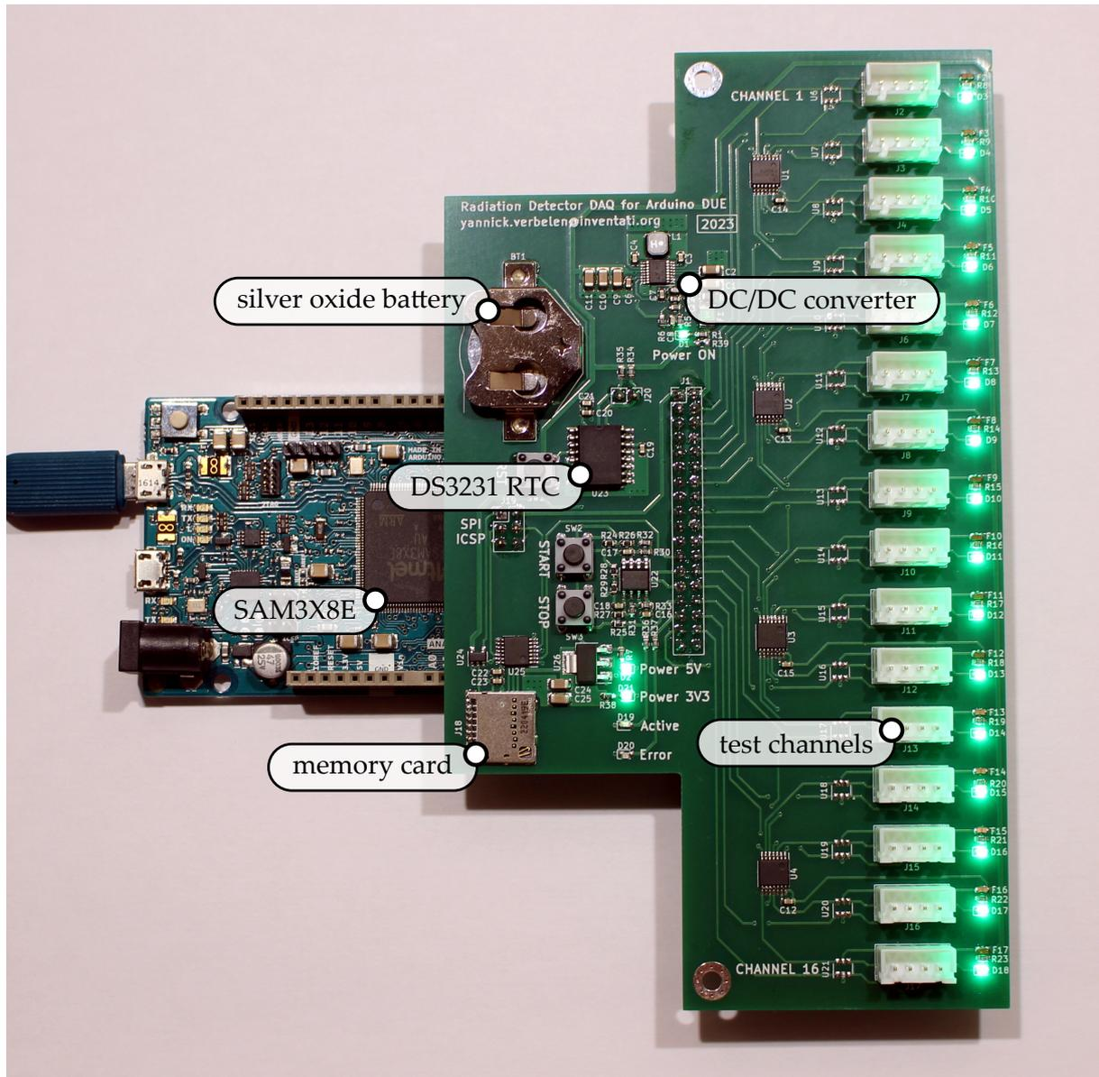
Figure 6: Prototype of the data acquisition system, showing the Arduino DUE microcontroller board (blue) and bespoke data acquisition card mounted on top (green). Channels 1 to 16 and their respective connectors are visible to the right.
