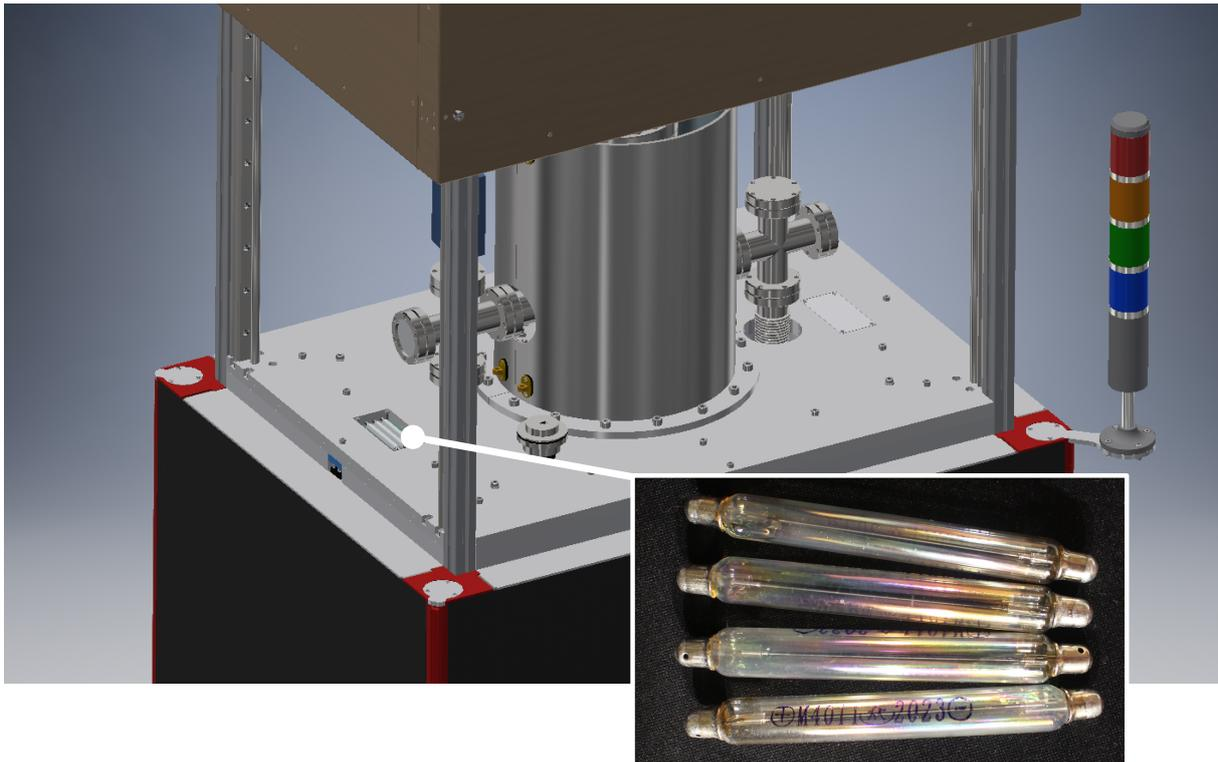
Figure 2: Location of the Geiger-Müller tube arrays of type M4011 [27] within the shielded environment of the particle accelerator. Radiation shields (brown) raised for clarity.
