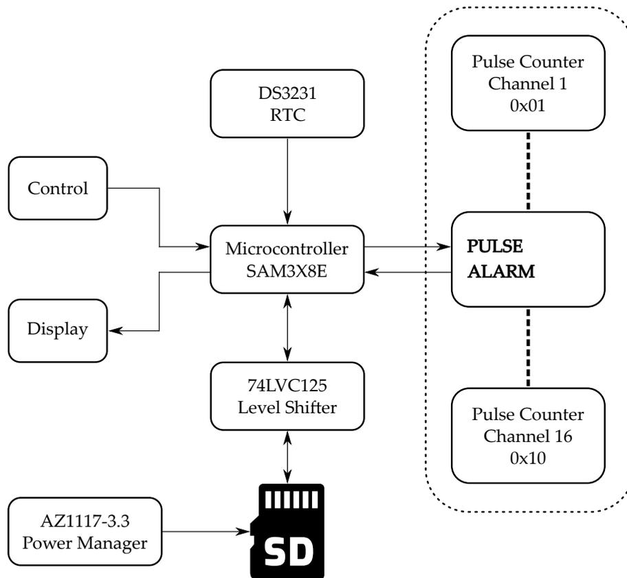
Figure 5: Block diagram of the data acquisition system with important components identified.
