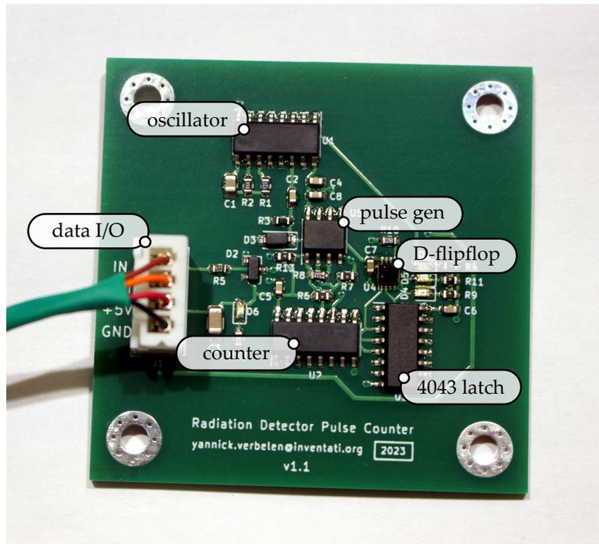
Figure 4: Prototype of the pulse counter designed and assembled, ready for radiation tolerance testing.
