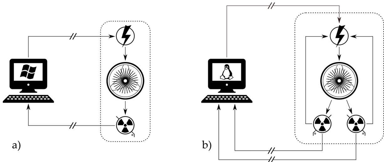
Figure 1: a) Quasi open-loop radiation control system found in a legacy commercial IECF device, relying on external software controls using unsuitable non-real-time operating systems to implement basic radiation protection. [26] b) Improved closed-loop radiation protection system for B34 interfacing directly with power supply and radiation shield actuation systems, featuring redundancy and resilience against external disruptions. [4]
