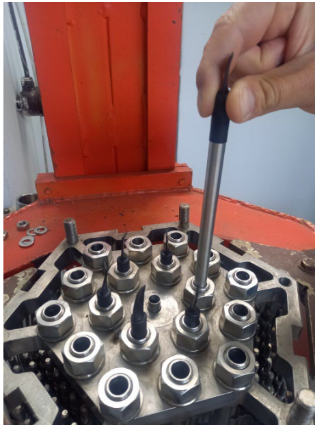
Figure 4: Insertion of absorber tubes into the inner row of the fuel assembly.
