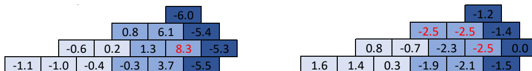
Figure 3: Deviations (%) from the reference of the normalized neutron flux distributions for the SP 3 solvers of FENNECS (left) and DYN3D (right) with 6 radial elements per assembly. The red numbers are the maximum deviations.
