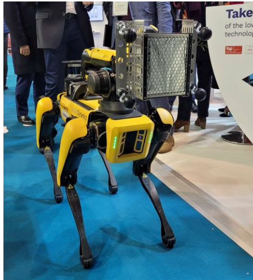
Figure 6: Autonomous robot carrying contamination probe presented at WNE 2021.
