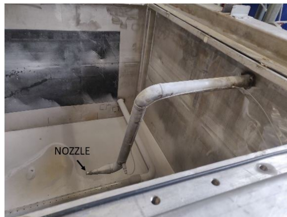
Figure 2: Nozzle of the experimental rig
