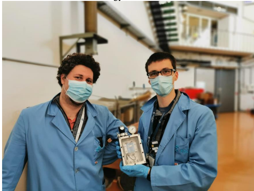
Figure 2: SiC neutron detector, that was tested inside the dry chamber facility at JSI TRIGA research reactor.
