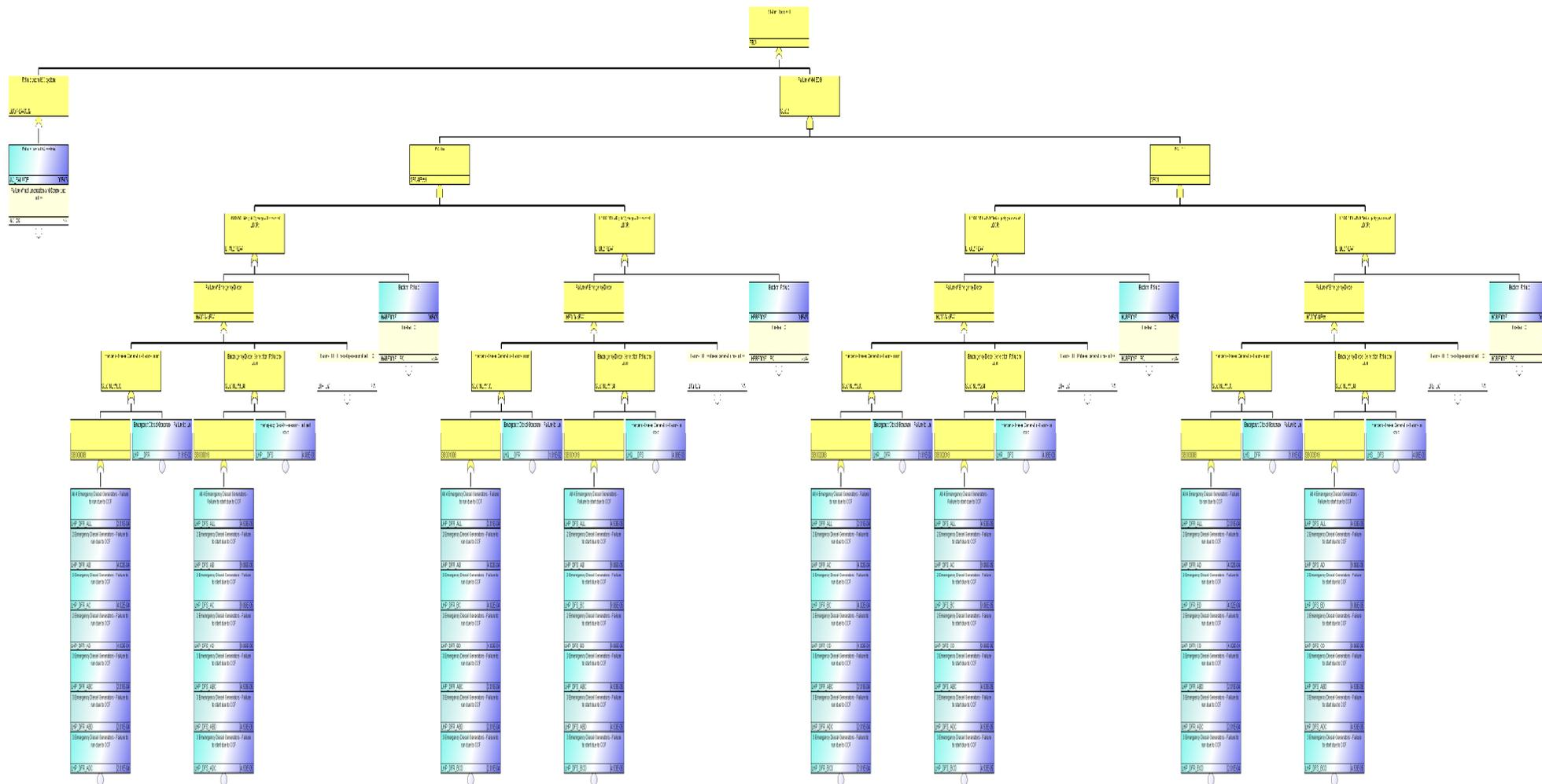
Figure 3 SBO Fault Tree without flooded components
