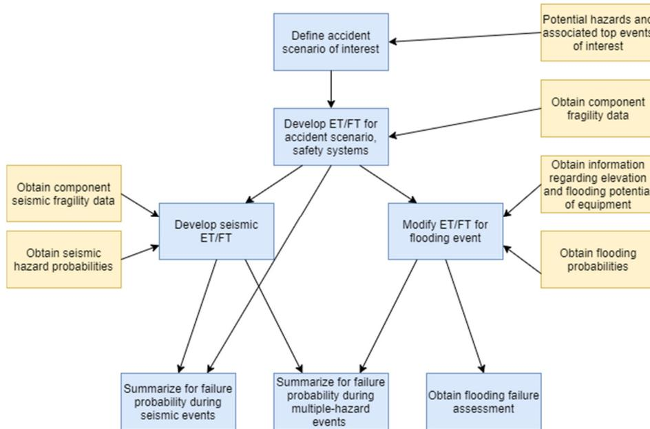
Figure 1 General methodology for multiple-hazard Probabilistic Safety Assessment: seismic and flooding
