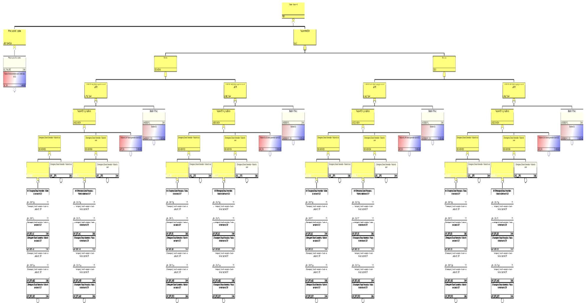
Figure 5 Example of SBO seismic fault tree
