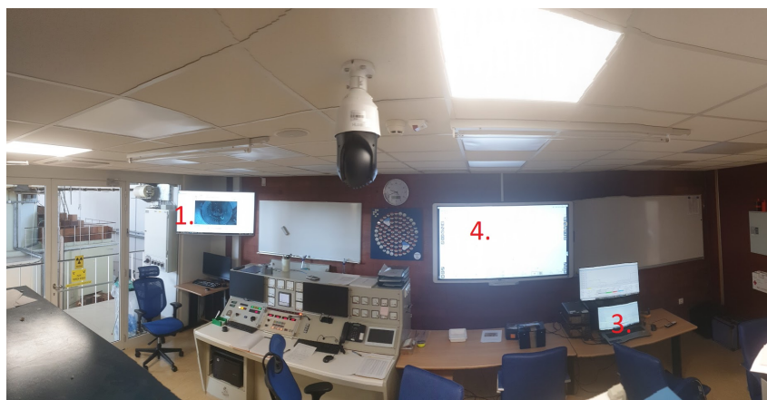
Figure 3: The dome camera is mounted on the ceiling and positioned so it can see the reactor control panel, nuclear instrumentation readings and a lecturer in front of the shared whiteboard
