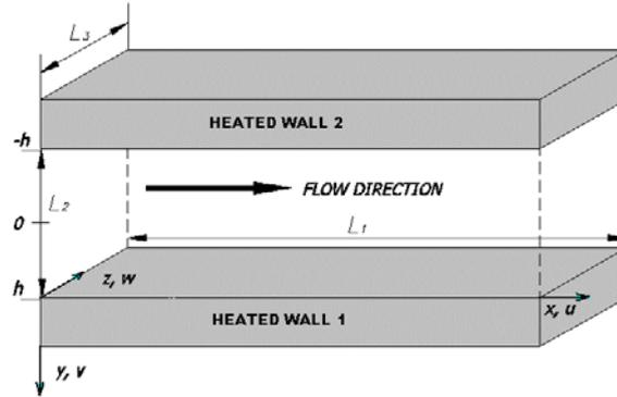
Figure 1: Computational domain.  $x$ ,  $y$  and  $z$  mark the three directions of coordinate axes, while  $u$ ,  $v$  and  $w$  mark the components of velocity. Flow is directed toward the positive  $x$  axis.
