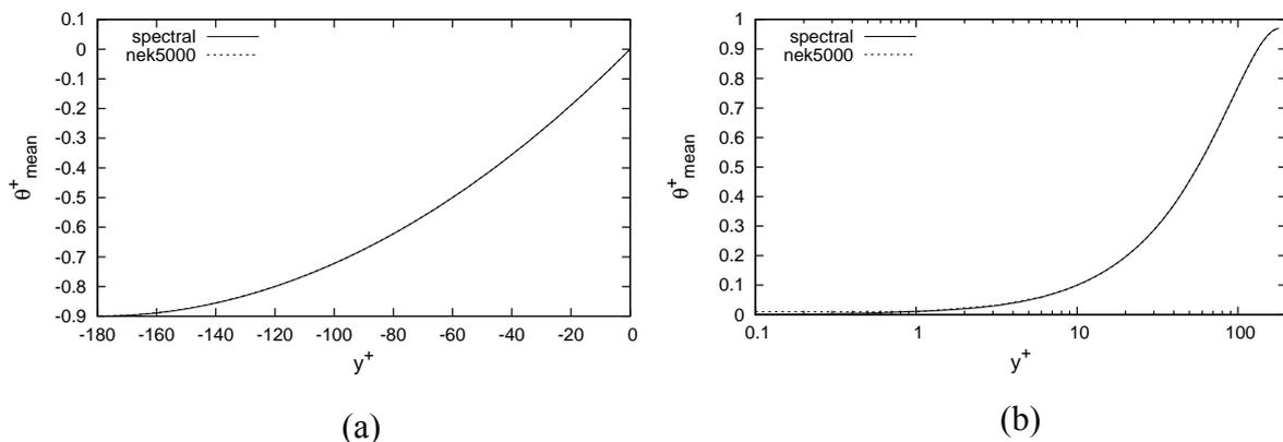
Figure 4: Mean temperature profiles in solid (a) and fluid (b).
