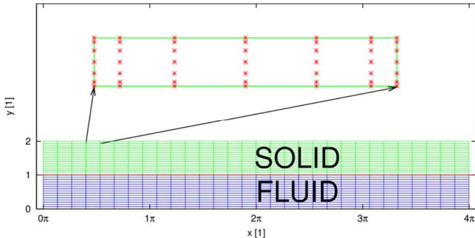
Figure 2: Bottom: half of the computational domain (2D projection) divided into spectral elements. Top: one spectral element of the 6th order (2D projection) with GLL points.
