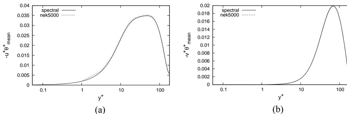
Figure 6: Streamwise (a) and wall-normal (b) turbulent heat fluxes.
