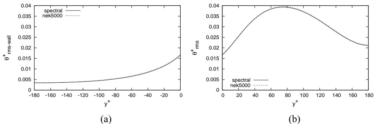
Figure 5: Temperature RMS fluctuations profiles in solid (a) and in fluid (b).
