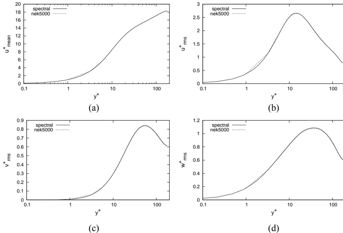
Figure 3: Comparison between spectral element scheme (Nek5000) and spectral scheme: (a) mean velocity, and (b, c, d) RMS fluctuations of components of velocities.
