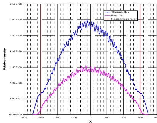
Fig. 6. Results from the Atucha-2 MCNP5 3D model – Thermal and Fast Flux distribution.
