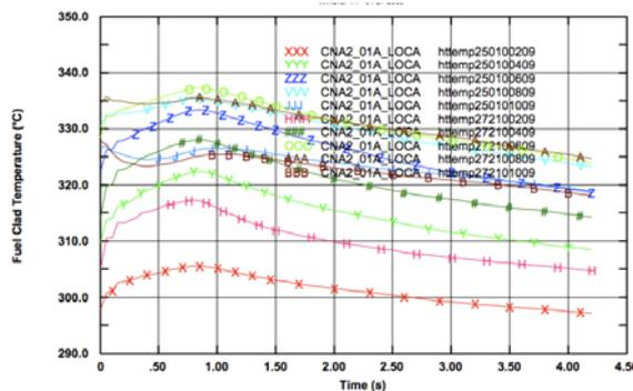
Fig. 13. Fuel Clad temperatures for Central and Hot Channel
