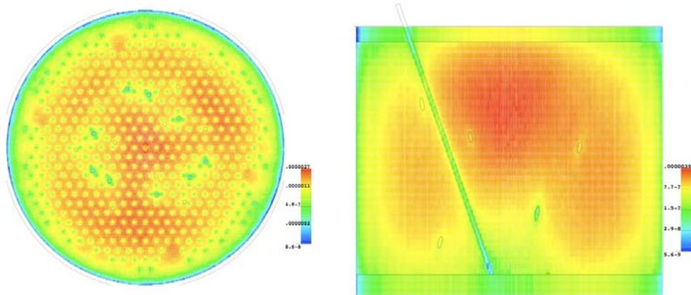
Fig. 5. Results from the Atucha-2 MCNP5 3D model – Thermal Flux distribution, planar and axial view.
