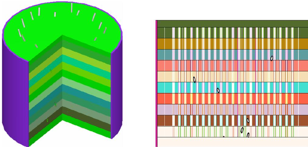
Figure. 4. Atucha-2 KENO-VI and MCNP5 models, ten level of axial detail.
