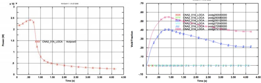
Fig. 12. Reactor Power (W) and void Fraction in central and hot channel
