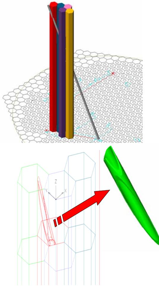
Fig. 7. Sketch of a CR and its crossing with 3D NK hexagonal cells.
